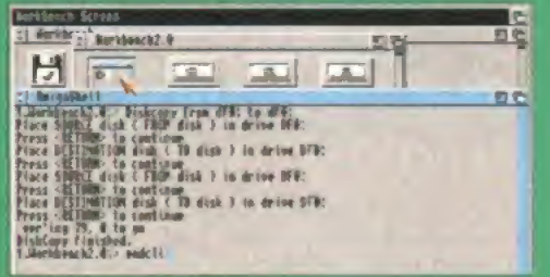
5 Put the source disk and destination disk in a couple more times when the Amiga asks for them. When it says "Diskcopy Finished" just type in: endcli to get out of the Shell or CLI. You may have to put the Workbench disk in again. Now your copy is ready!
